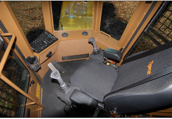
Rotating seat with joystick steering. Better ergonomics and reduced neck strain.
