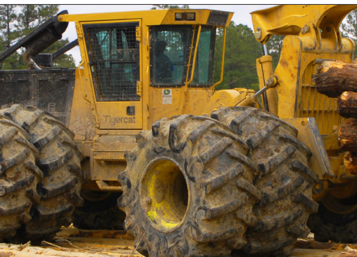
All E-series models are standard equipped for dual or flotation tires.
