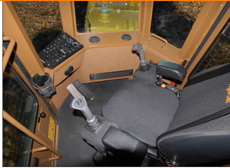
Turnaround provides full rear-facing controls for reduced neck strain when travelling grapple-forward, gathering a bunch or performing decking duties.
