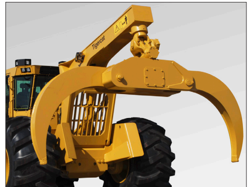
High capacity dual cylinder grapple options.
